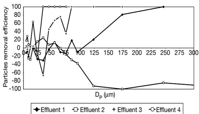
**Figure 2.** Efficiency of a 130 µm disc filter (D130) at removing different particle sizes (Dp) from effluents.
