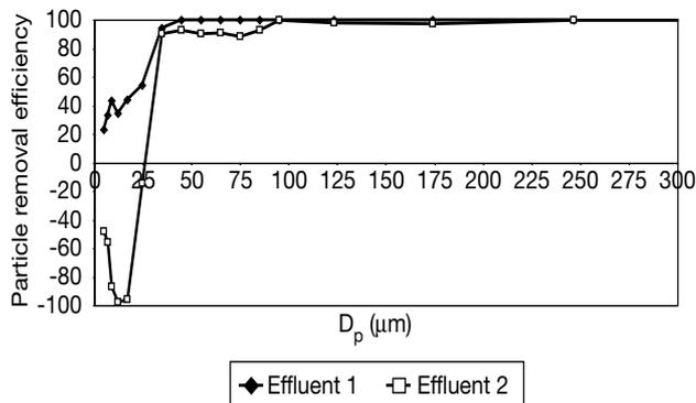
**Figure 4.** Efficiency of sand filter at removing different particle sizes (Dp) from Effluents 1 and 2.
