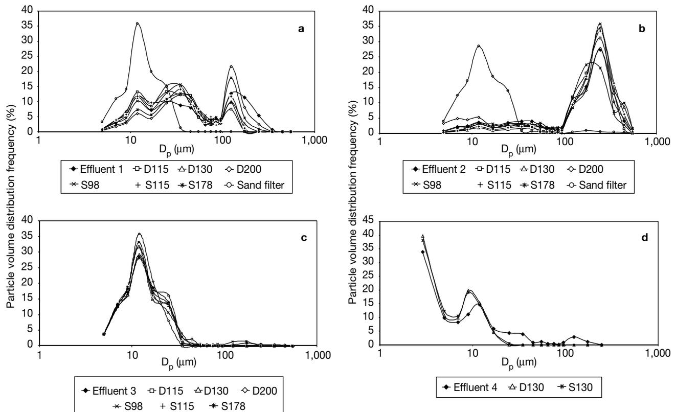
**Figure 5.** Mean particle volume distributions of Effluent 1 (a), 2 (b), 3 (c) and 4 (d) before and after filtration with a 115  $\mu\text{m}$  (D115), 130  $\mu\text{m}$  (D130) and 200  $\mu\text{m}$  (D200) disc filter, 98  $\mu\text{m}$  (S98), 115  $\mu\text{m}$  (S115) and 178  $\mu\text{m}$  (S178) screen filter, and a sand filter with an effective grain size of 0.65 mm.
