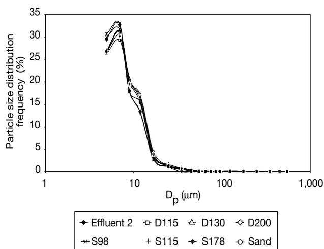
**Figure 1.** Mean particle size distributions of the secondary effluent from the Girona wastewater treatment plant (Effluent 2) before and after filtration with 115  $\mu\text{m}$  (D115), 130  $\mu\text{m}$  (D130) and 200  $\mu\text{m}$  (D200) disc filters, 98  $\mu\text{m}$  (S98), 115  $\mu\text{m}$  (S115) and 178  $\mu\text{m}$  (S178) screen filters, and a sand filter with a 0.65 mm effective grain size.
