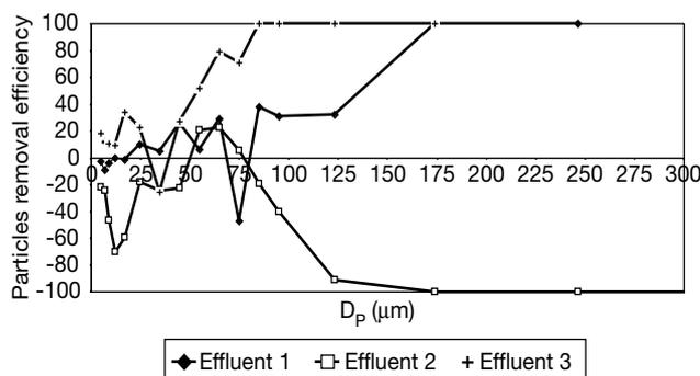
**Figure 3.** Efficiency of a 115 µm screen filter (S115) at removing different particle sizes (Dp) from effluents.
